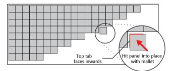
Do not directly hit the edge of the **GenieMat FF** panels with a mallet or hammer. Use a wood block flush with the edge to distribute the load and protect the edges as the panels are hit into place.
