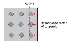
vi. Install cut panels around perimeter to complete grid.
