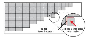
Do not directly hit the edge of the **GenieMat FF** panels with a mallet or hammer. Use a wood block flush with the edge to distribute the load and protect the edges as the panels are hit into place.
