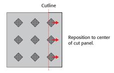
vi. Install cut panels around perimeter to complete grid.
