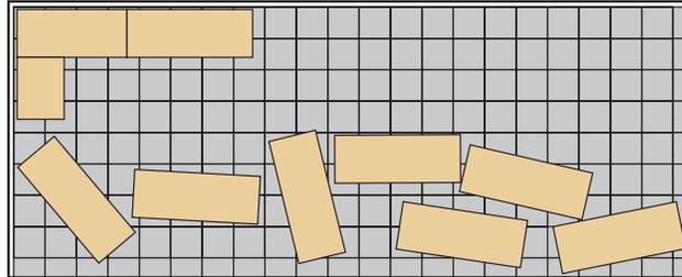
**ix.** Install the plywood offsetting the seams from the panels and adjacent layers of plywood. Screw the plywood every 12" on center (screw length should not exceed the thickness of the two layers being screwed together).
