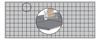
**viii.** Avoid walking on installed and stapled **GenieMat FF70/FF70LDM** panels. Place plywood on top in high traffic areas to prevent damaging the panels.
