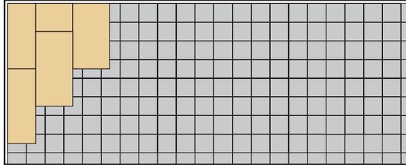
x. Nail or screw in a piece of plywood to bridge the perimeter gap. This will ensure no concrete seeps down into the gap. The 3 mil poly sheet is installed on top of this piece of plywood.
