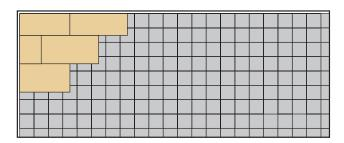
$\mathbf{x}.$  Repeat step 9 with second layer of plywood crosslaying in the opposite direction.
