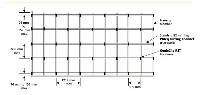
Wall or Ceiling Framing at 406 mm o.c. **GenieClip RST** at 1219 mm o.c., furring at 609 mm o.c. 1 or 2 Layers of 16 mm plasterboard
